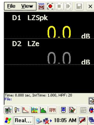
[Fig. IV-2-15] Display with various units in SLM
